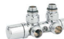
RXV421 Thermostatic mono/tube angle valve with by-pass and lockshield. Distance between connections 50 mm. / Robinet termostabil mono/bitubular de colț interax 50 mm.
